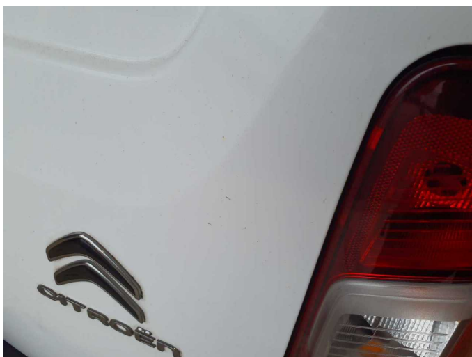
Damage 4: Body: Body (Flugrost) - Soiled - Conditioning
