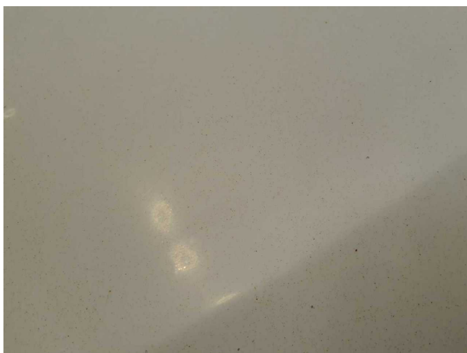
Damage 4: Body: Body (Flugrost) - Soiled - Conditioning
