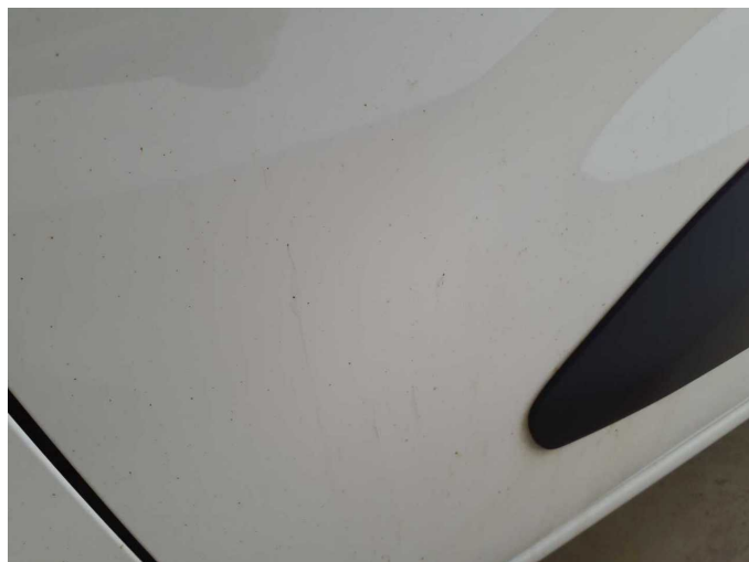
Damage 4: Body: Body (Flugrost) - Soiled - Conditioning
