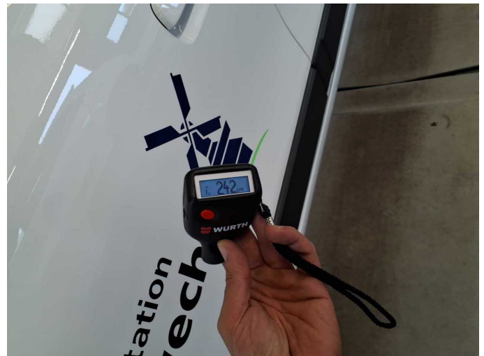
Repainting 1: Door - front left side
