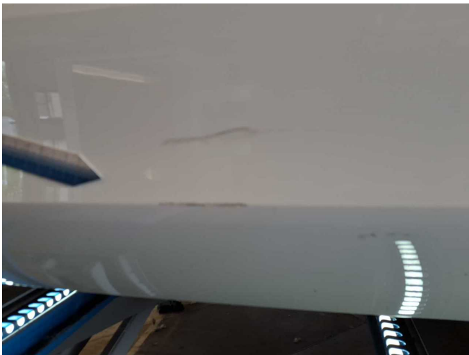
Damage 1: Rear bumper: Rear bumper - Scratch(es) - Smart repair
