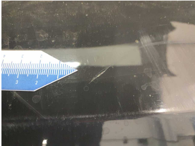
Damage 8: Rear bumper: Rear bumper - Scratch(es) - Paint
