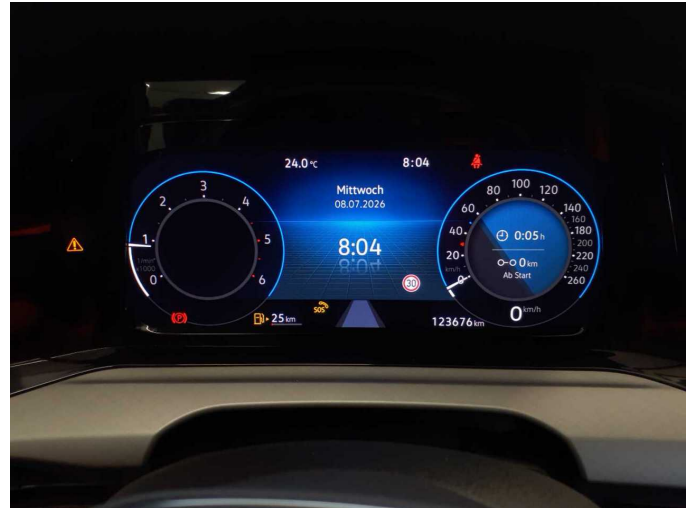
Damage 1: Instrument panel: Indicator light (Notruffunktion) - Specify findings - Perform diagnosis
