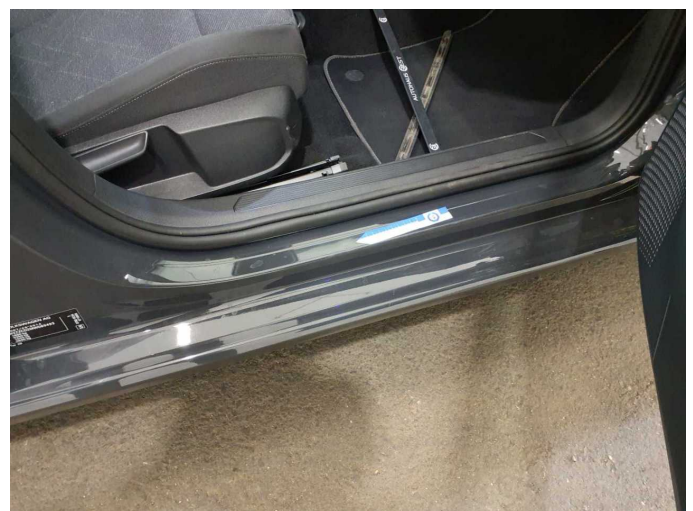
Damage 3: Sill - right side: Sill - dent(s) - Smart repair
