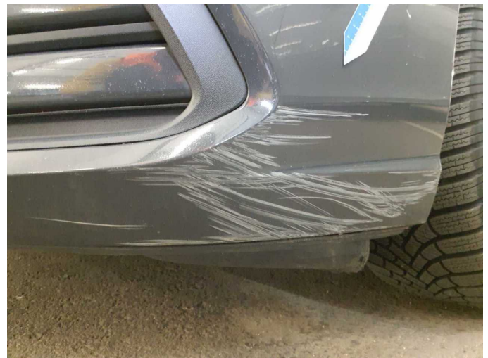
Damage 7: Front bumper: Front bumper - Scratch(es) - Paint
