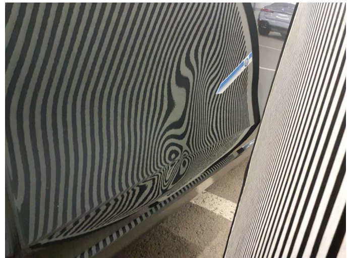
Damage 10: Door - front right side: Door - dent(s) - Repair and paint
