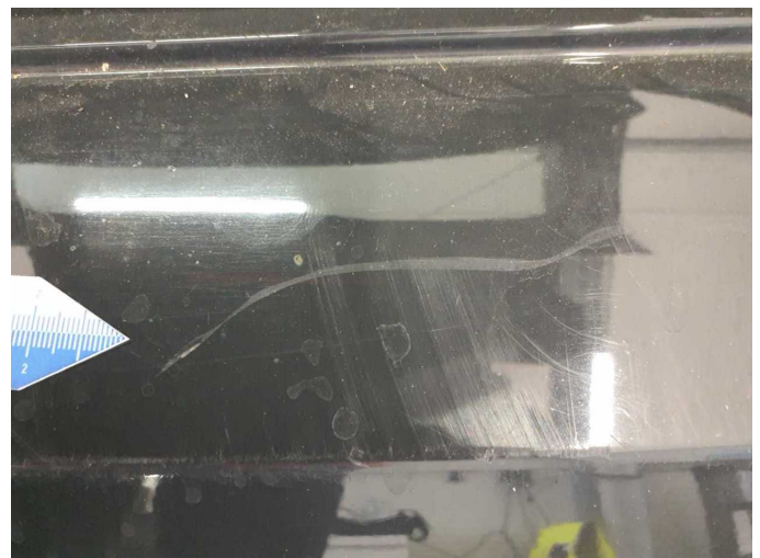
Damage 8: Rear bumper: Rear bumper - Scratch(es) - Paint
