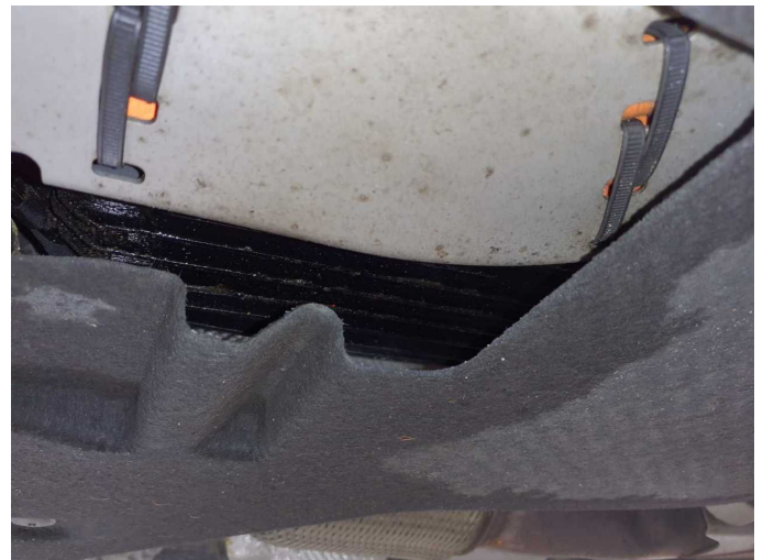
Damage 2: Gearbox: Gearbox (Ölverlust) - Leaking - Perform diagnosis
