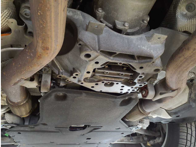
Damage 2: Gearbox: Gearbox (Ölverlust) - Leaking - Perform diagnosis
