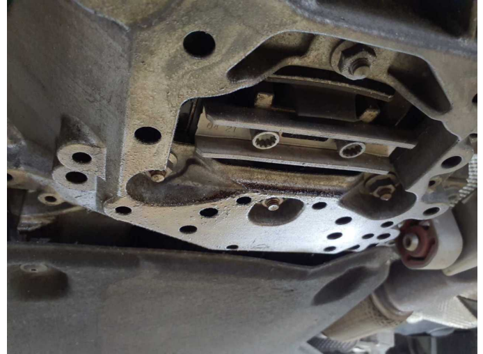
Damage 2: Gearbox: Gearbox (Ölverlust) - Leaking - Perform diagnosis
