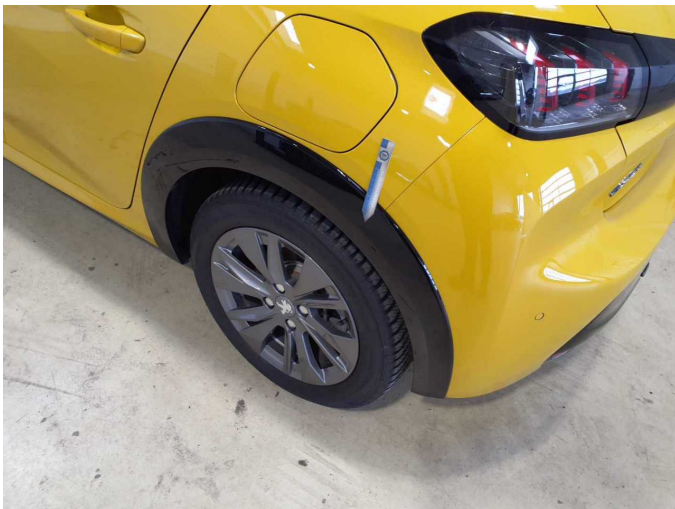
Damage 9: Side panel - rear left side: Wheel arch - Scratch(es) - Replace
