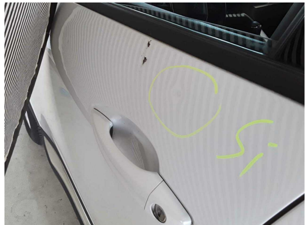
Damage #4: Door - front left side: Door - dent(s) - Smooth repair work
