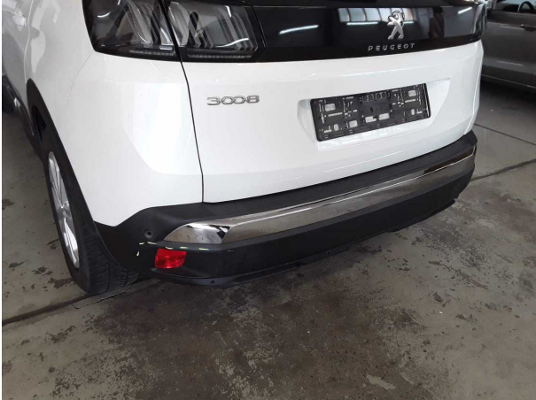
Damage #3: Rear bumper: Spoiler - Scratched - Loss in value
