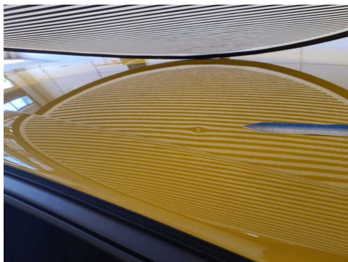
Damage 1: Roof: Roof - dent(s) - Smooth repair work
