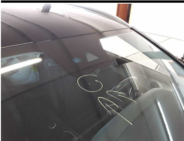
Damage #4: Vehicle glazing: Windscreen (Rissbildung) - Stone chips - Replace
