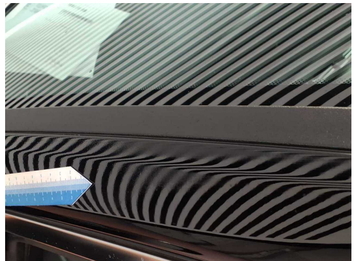
Damage 5: Roof: Roof rail - left side (Wellig) - Unprofessionally repaired - Paint
