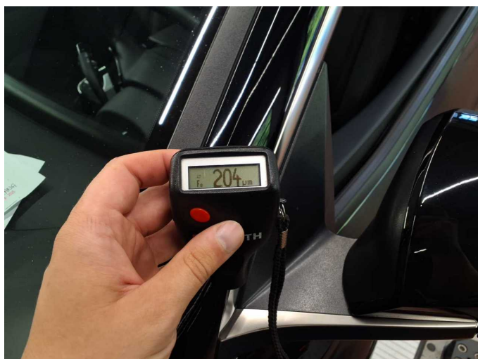
Repainting 1: Roof rail - left side
