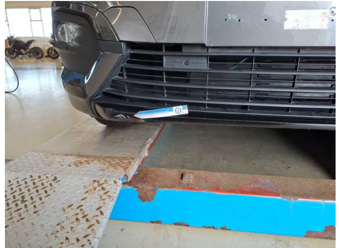
Damage 2: Trim / covers: Trim / covers (Stoßfänger vorn) - Scratch(es) - Smart repair
