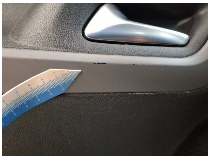
Damage 8: Trim / covers: Door trim - front left side - Scratched - Replace
