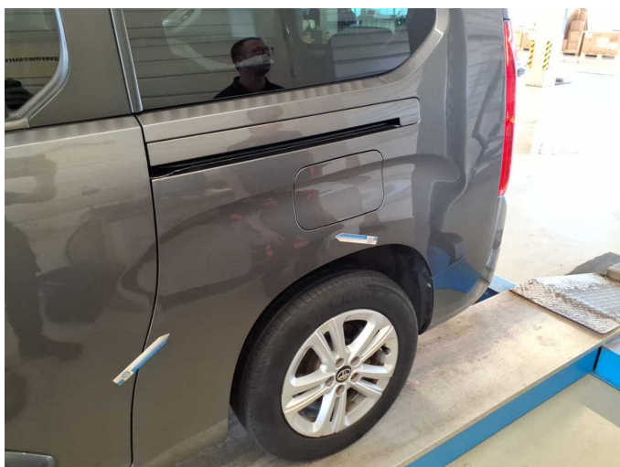
Damage 11: Side panel - rear left side: Side panel (wellig-teilweise) - Unprofessionally repaired - Repair and paint
