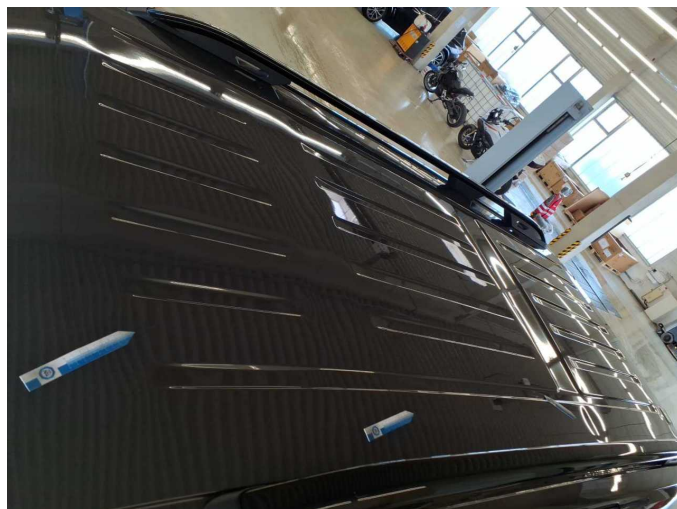
Damage 6: Roof: Roof - dent(s) - Smooth repair work
