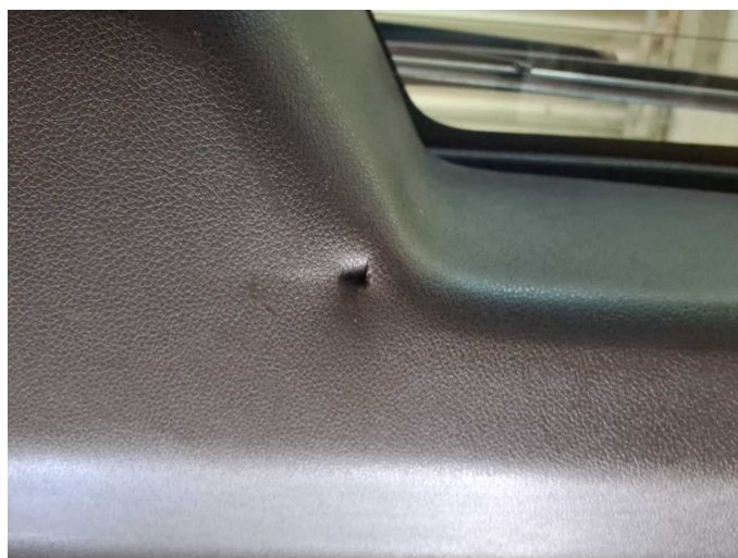
Damage 9: Boot lid / rear door: Trim - standard - lower - Broken / torn - Replace
