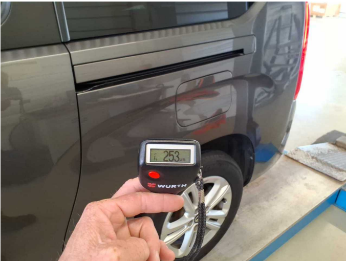
Side panel - rear left side: 253 µm
