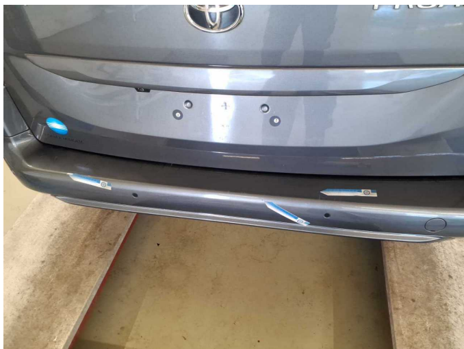
Damage 10: Rear bumper: Bumper with Parktronic - Scratched - Paint
