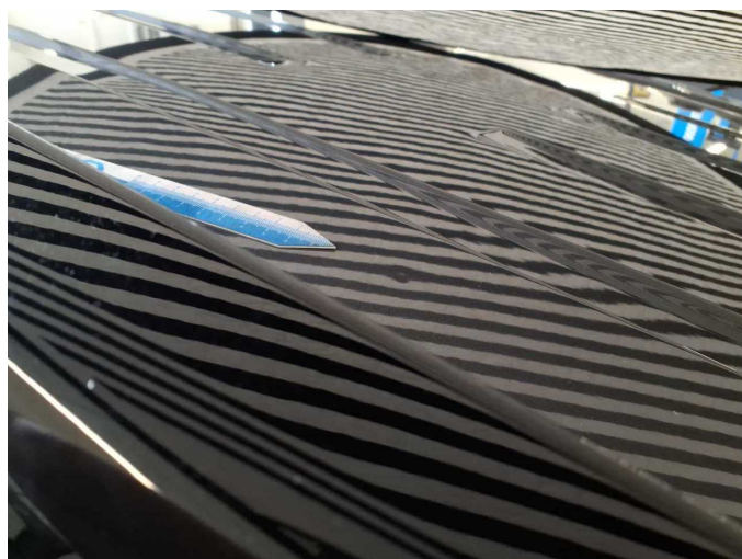
Damage 6: Roof: Roof - dent(s) - Smooth repair work
