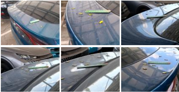
Roof, Hail damage, Repair and paint (complete)
