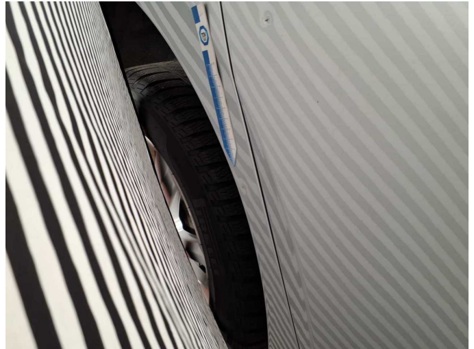
Damage 11: Side panel - rear right side: Elbow - Dent / paintcoat damage - Paint
