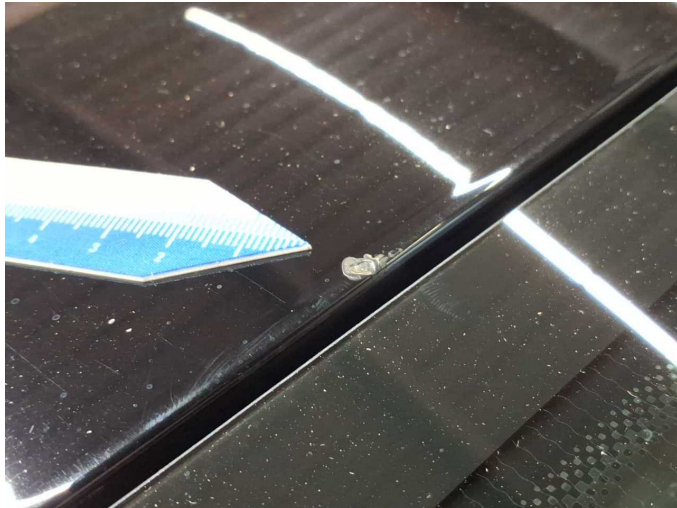
Damage 15: Roof: Roof - Stone chips - Paint
