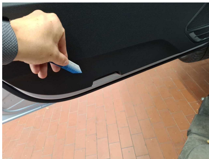
Damage 1: Trim / covers: Door trim - front left side (Rückstrahler) - Missing - Replace
