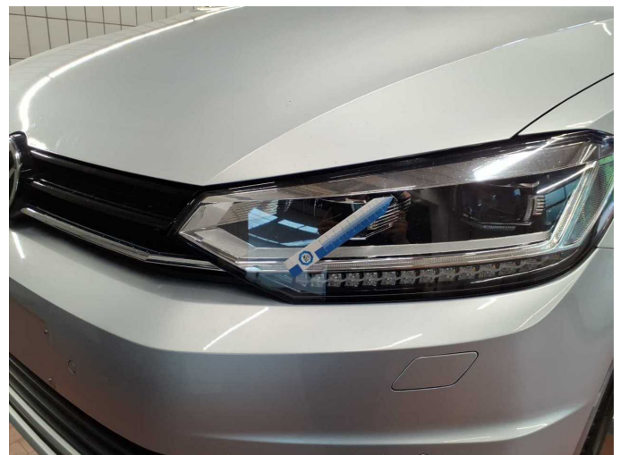
Damage 14: Headlight: Headlight - left side - Scratch(es) - Replace
