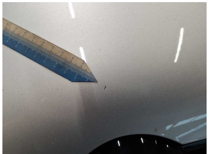
Damage 12: Bonnet: Bonnet - Stone chips - Paint
