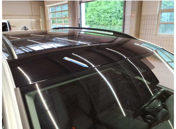
Damage 15: Roof: Roof - Stone chips - Paint
