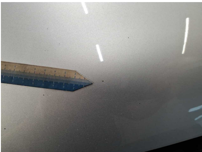
Damage 12: Bonnet: Bonnet - Stone chips - Paint
