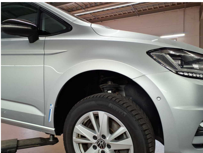
Damage 4: Mudguard - right side: Mudguard - right side - Scratch(es) - Smart repair
