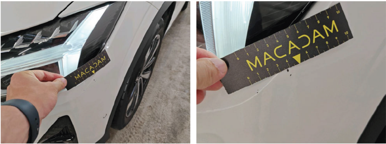
Bumper F Stone chip(s) Repair and paint (complete) Front
