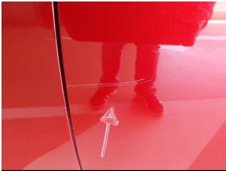
Tür / Hinten Links / Kratzer
