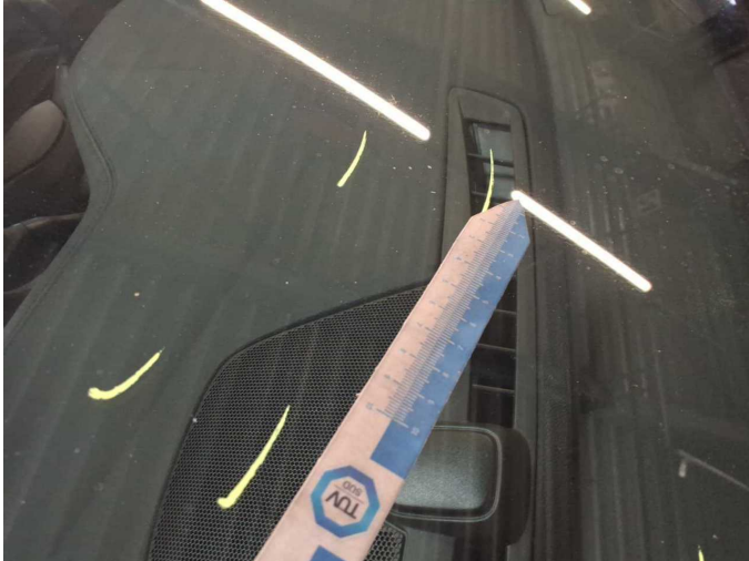
Damage 7: Vehicle glazing: Windscreen - Stone chips - Replace
