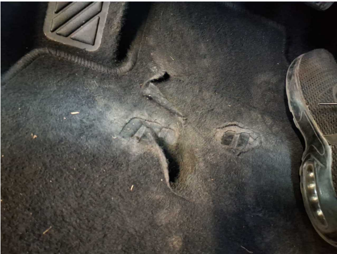
Damage 1: Trim / covers: Floor mats (Vorne links) - Holes - Replace
