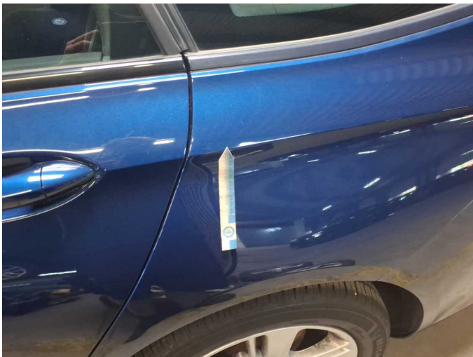
Wear and tear 1: Side panel - rear left side: Side panel - dent(s) - No deduction
