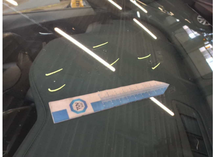
Damage 7: Vehicle glazing: Windscreen - Stone chips - Replace
