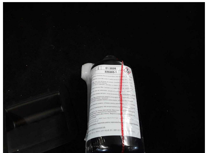
Damage 1: Equipment: Tirefit filler - Expired - Replace
