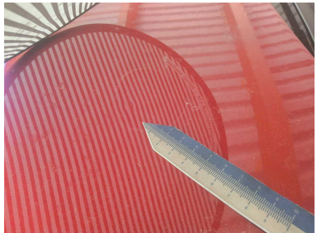
Damage 1: Bonnet: Bonnet - dent(s) - Smooth repair work
