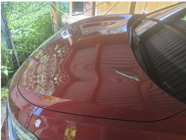
Damage 1: Bonnet: Bonnet - dent(s) - Smooth repair work
