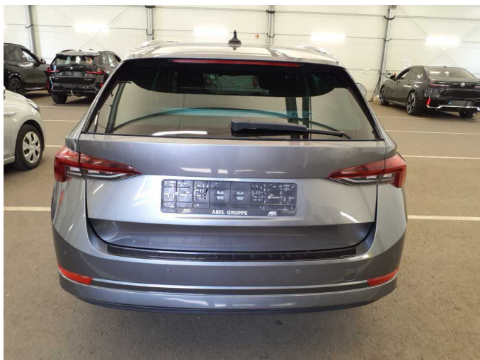
Damage 3: Boot lid / rear door: Lettering - Missing - Replace
