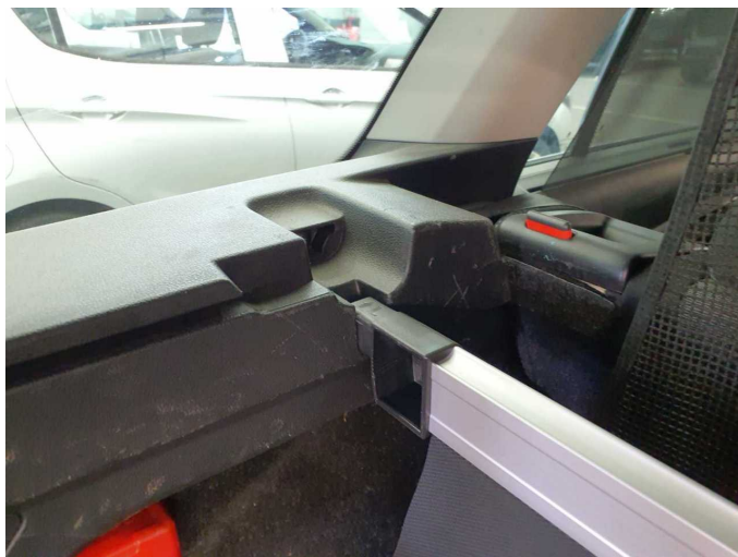
Missing part 4: Interior: Boot cover / roller cover - Missing - Replace
