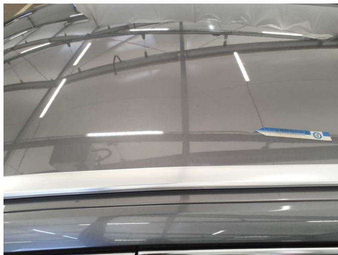
Damage 4: Roof: Roof - dent(s) - Smart repair
