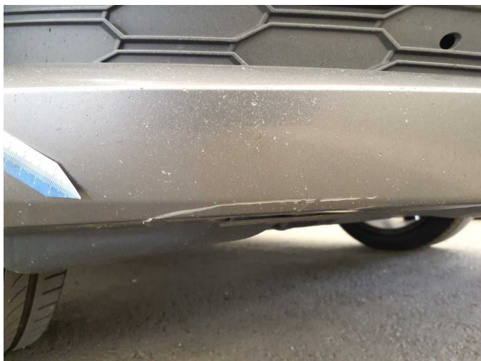
Damage 6: Front bumper: Front bumper - Scratch(es) - Paint
