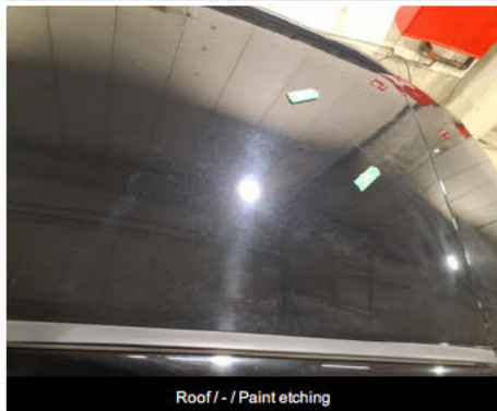
Roof / - / Paint etching
