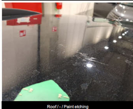
Roof / - / Paint etching
