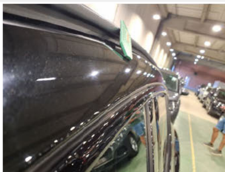
Roof post A/B/C / Left / Dent
