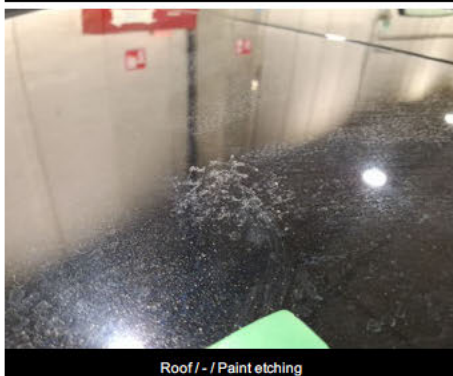
Roof / - / Paint etching
