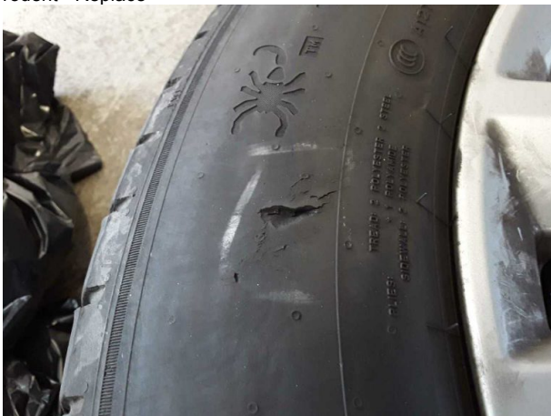
Damage #5: 2nd wheel set: 1 tyre - Damaged - Replace
