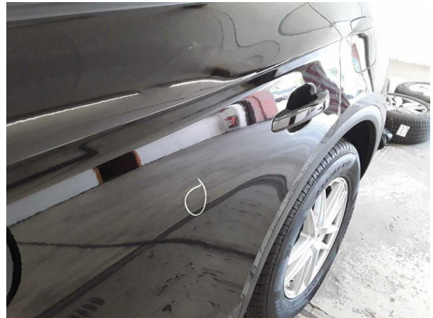
Damage #3: Door - rear left side: Door - dent(s) - Smooth rep... work
