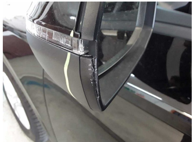
Damage #6: Wing mirror - left side: Mirror housing - Scratches... Replace
