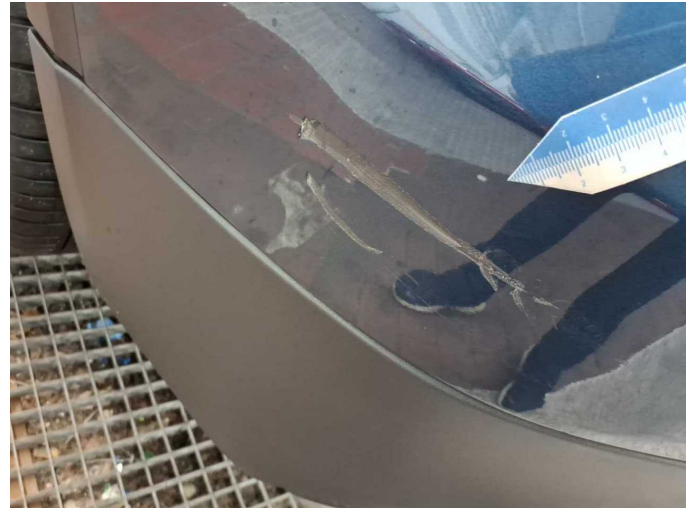
Damage 4: Rear bumper: Rear bumper - Dent / paintcoat damage - Repair and paint
