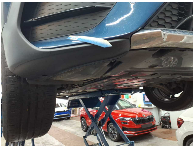
Damage 3: Front bumper: Spoiler (Zierleiste re) - Broken / torn - Replace
