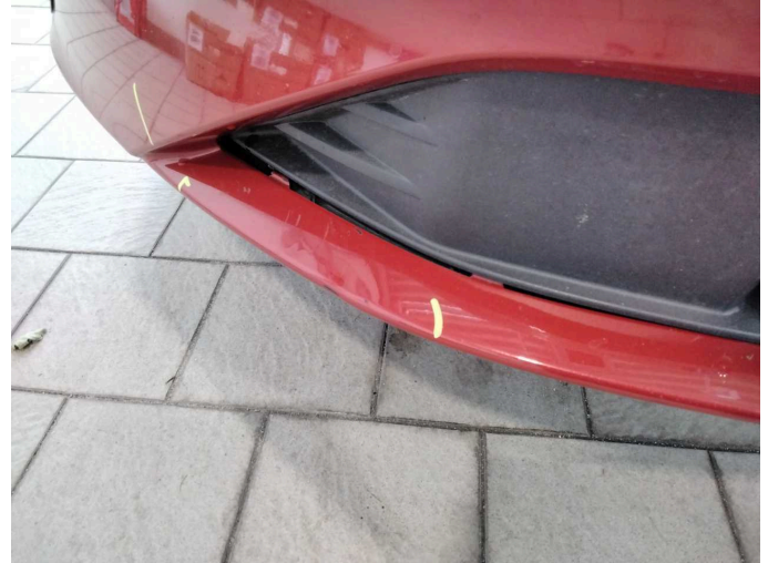
Damage 1: Front bumper: Front bumper - Malposition - Set / adjust
