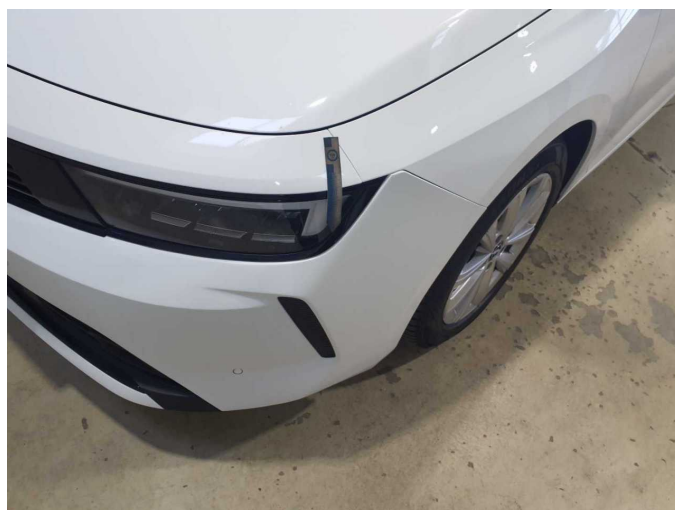
Damage 7: Trim / covers: Trim / covers (Scheinwerfer zierleiste) - Scratch(es) - Replace
