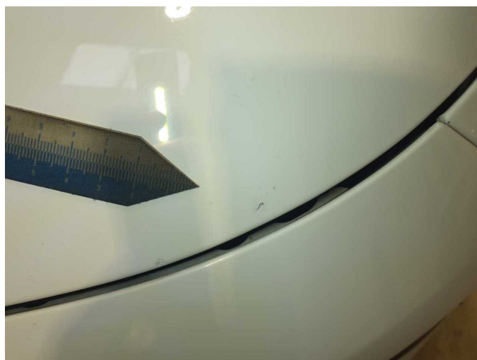
Damage 11: Bonnet: Bonnet - Scratch(es) - Paint
