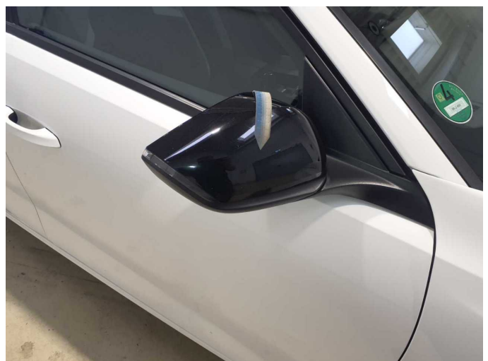
Damage 1: Wing mirror - right side: Cap (Lack nebel) - Paint defect - Smart repair
