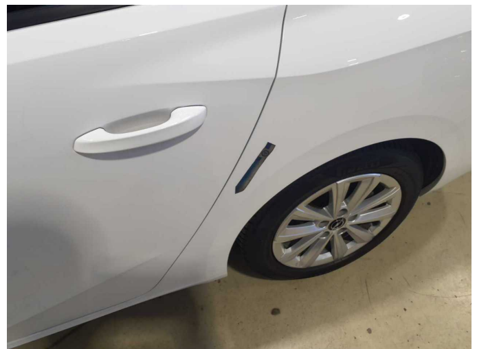
Damage 10: Side panel - rear left side: Side panel (Wellig) - Unprofessionally repaired - Paint
