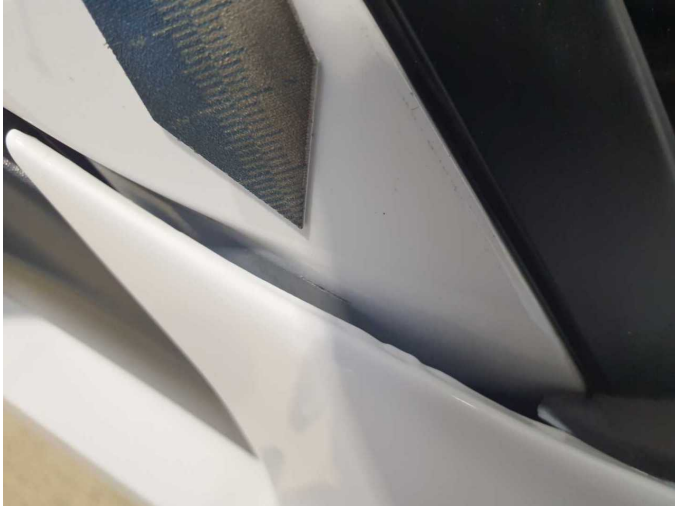
Damage 8: Body: A-pillar - right side (Lack nebel) - Paint defect - Paint
