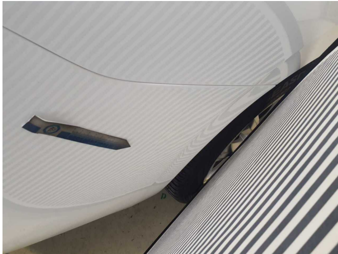
Damage 12: Rear bumper: Rear bumper - dent(s) - Paint
