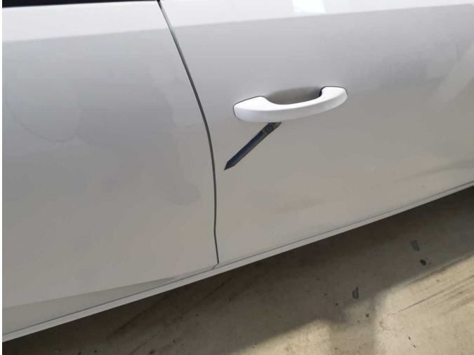
Damage 4: Door - front right side: Door edge - Dent / paintcoat damage - Smart repair
