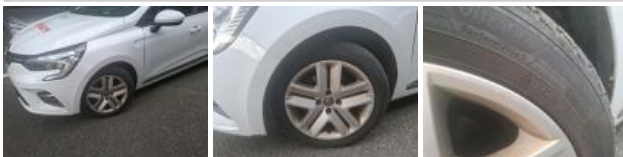
Tyre RL, Out of tolerance, Replace
