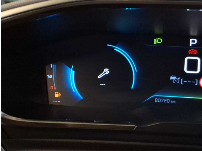
Damage 3: Misc.: Inspection / maintenance - Due - Perform
