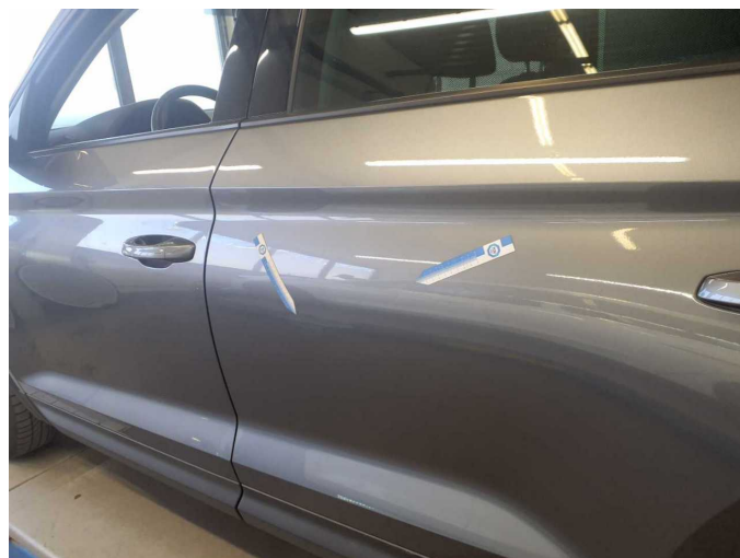
Damage 3: Door - rear left side: Door (3) - dent(s) - Smart repair
