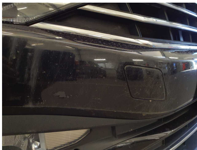
Damage 5: Front bumper: Front bumper - Scratch(es) - Paint
