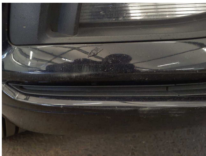
Damage 5: Front bumper: Front bumper - Scratch(es) - Paint
