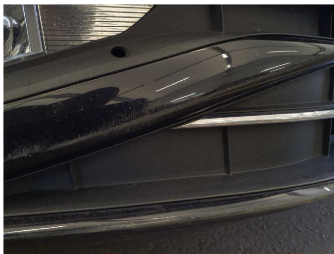
Damage 5: Front bumper: Front bumper - Scratch(es) - Paint
