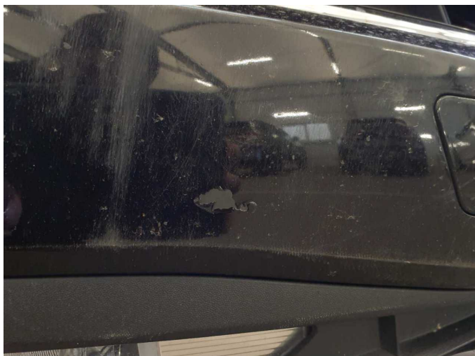
Damage 5: Front bumper: Front bumper - Scratch(es) - Paint
