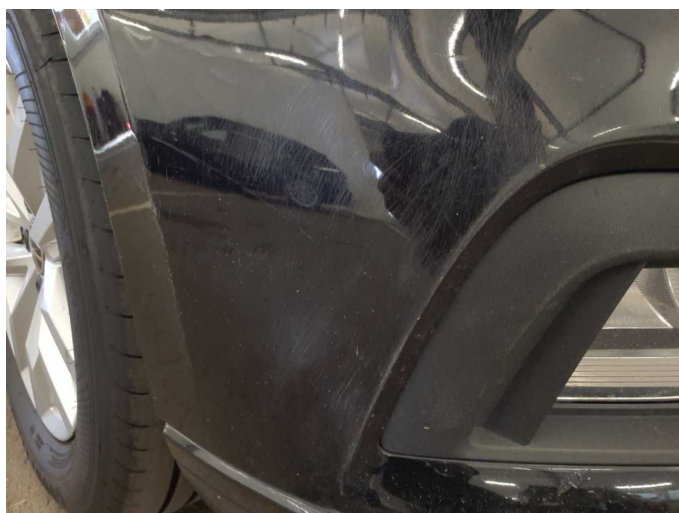
Damage 5: Front bumper: Front bumper - Scratch(es) - Paint
