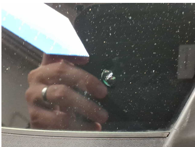
Damage 4: Vehicle glazing: Windscreen - Stone chips - Replace
