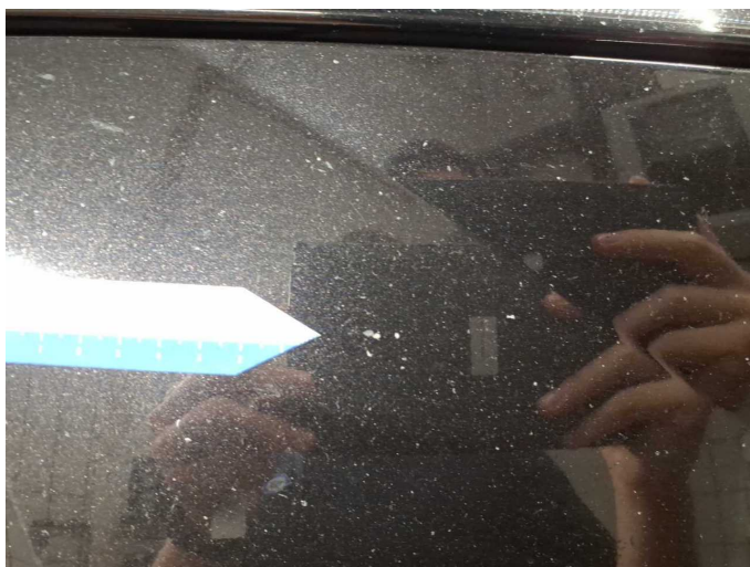
Damage 2: Front bumper: Front bumper - Stone chips - Paint
