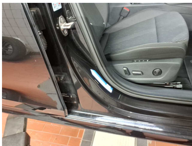
Damage 1: Sill - right side: Sill - Scratch(es) - Smart repair
