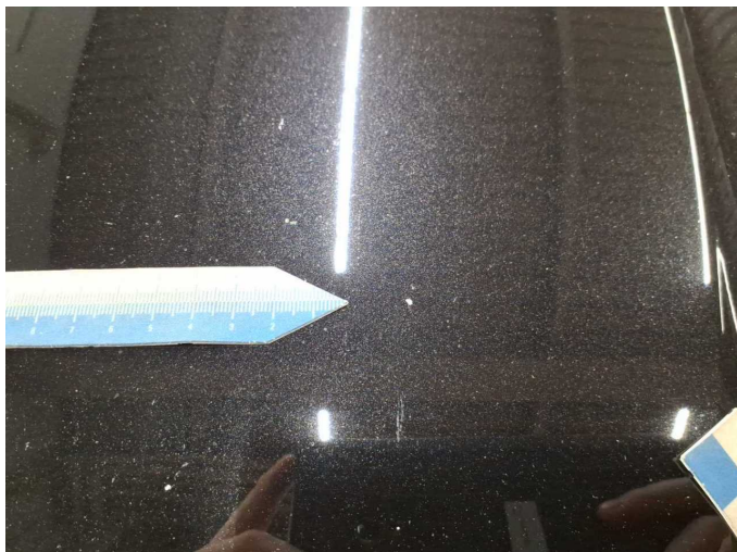
Damage 3: Bonnet: Bonnet - Stone chips - Paint
