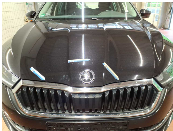
Damage 3: Bonnet: Bonnet - Stone chips - Paint
