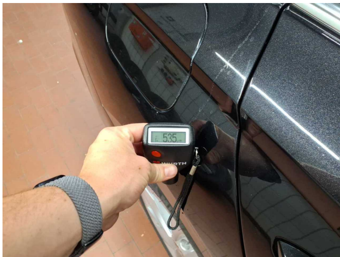
Repainting 1: Side panel - rear right side
