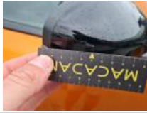
Outside rear-view mirror housing R, Scratch(es), Acceptable
