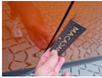
Outside rear-view mirror housing R, Scratch(es), Acceptable
