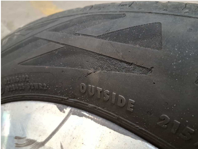
Damage 1: 2nd wheel set: 2 tyres (Flanke Sommerreifen) - Damaged - Replace
