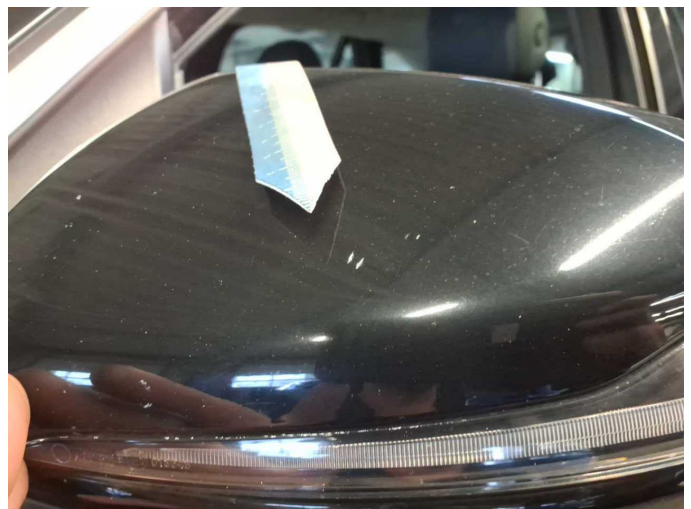
Damage 2: Wing mirror - left side: Cap - Stone chips - Smart repair
