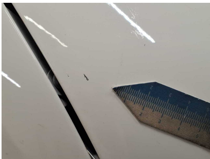
Damage 4: Bonnet: Bonnet - Stone chips - Repair and paint
