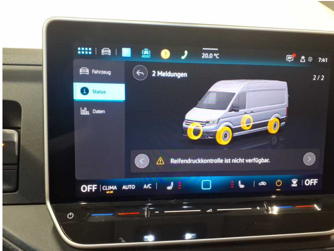
Damage 2: Electronic systems: Electronic systems (Reifendruckkontrollsystem) - Electrical fault - Perform diagnosis
