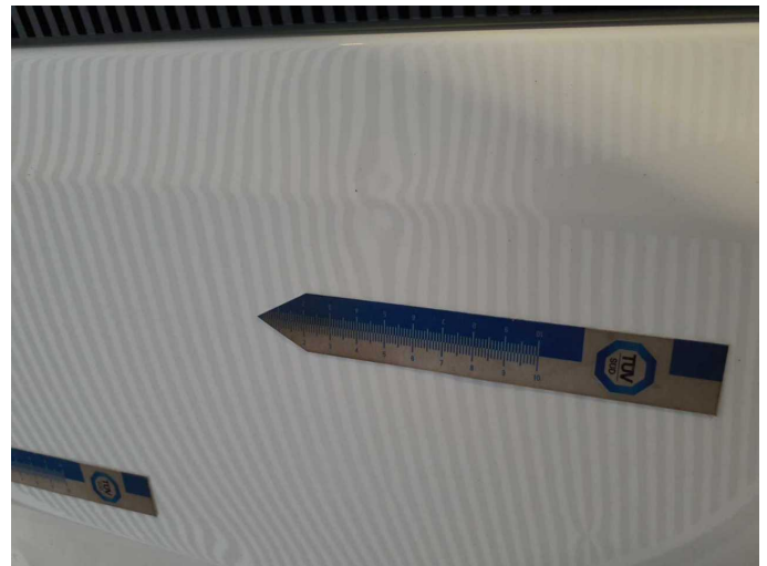
Damage 6: Sliding door, right: Sliding door - dent(s) - Smart repair
