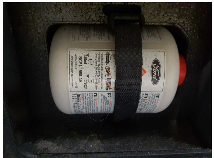
Damage 1: Equipment: Tirefit filler - Expired - Replace
