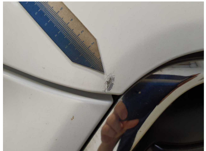
Damage 4: Bonnet: Bonnet - Scratch(es) - Smart repair
