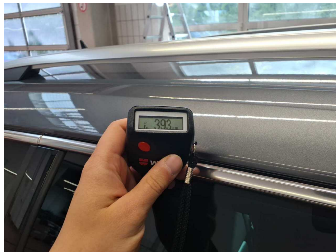
Repainting 4: Roof rail - right side
