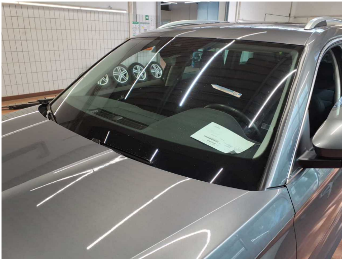
Wear and tear 3: Vehicle glazing: Windscreen (Ohne Rissbildung) - Stone chips - No deduction
