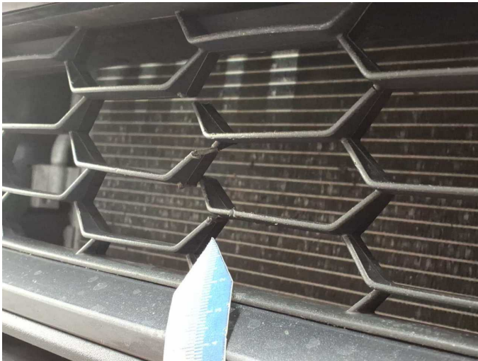
Damage 3: Front bumper: Grille - Broken / torn - Replace
