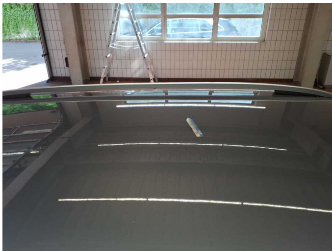
Damage 5: Roof: Roof (Lackeinschlüsse; wellig (+Dellen Gebrauchspur)) - Unprofessionally repaired - Paint
