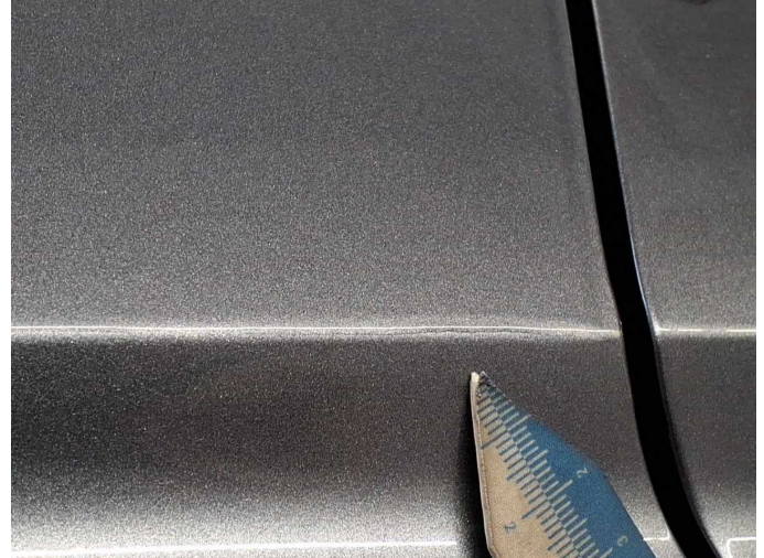
Damage 4: Side panel - rear right side: Side panel (Lackeinschlüsse, Lackierkante sichtbar) - Unprofessionally repaired - Paint
