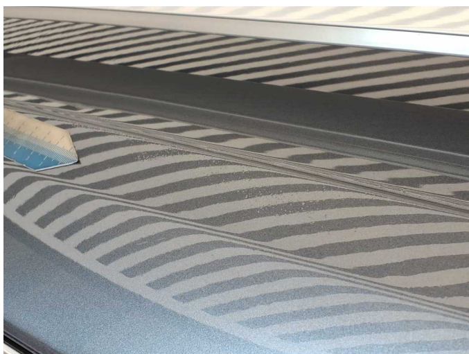
Damage 1: Roof: Roof rail - left side (Lackeinschlüsse) - Unprofessionally repaired - Paint
