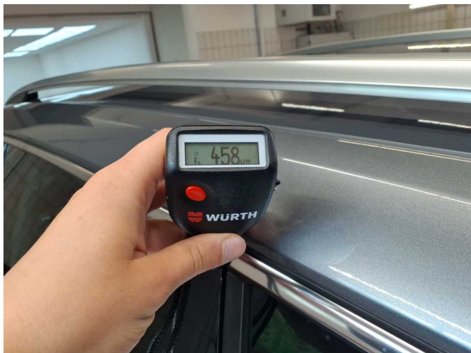
Repainting 3: Roof rail - left side
