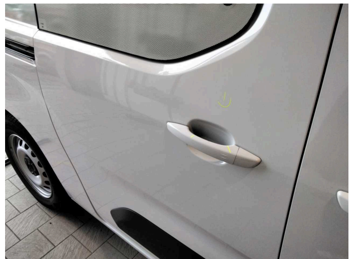
Damage 3: Door - rear right side: Door handle - outside - Scratch(es) - Smart repair
