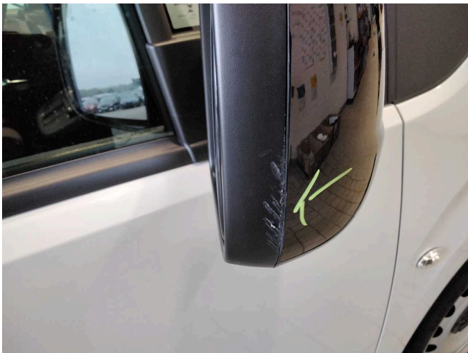
Damage 4: Wing mirror - right side: Mirror housing - Scratch(es) - Smart repair
