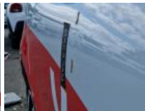
Wing RR, Dent(s), Repair and paint (complete)
