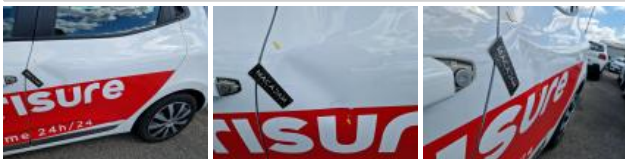
Outer door handle FL, Incomplete, Replace
