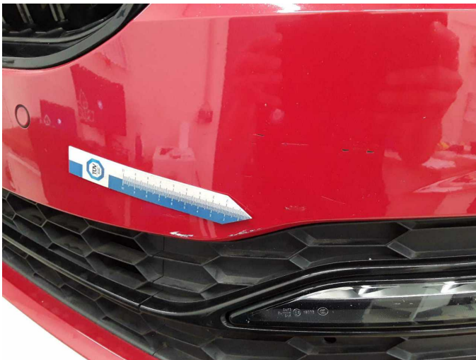
Damage 8: Front bumper: Front bumper - Scratch(es) - Paint
