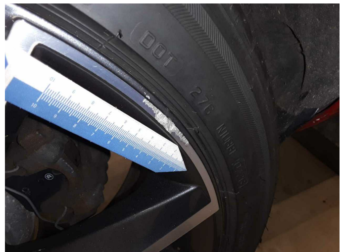
Wear and tear 2: Wheel / tyres: Alloy rim - rear right side - Scratch(es) - No deduction
