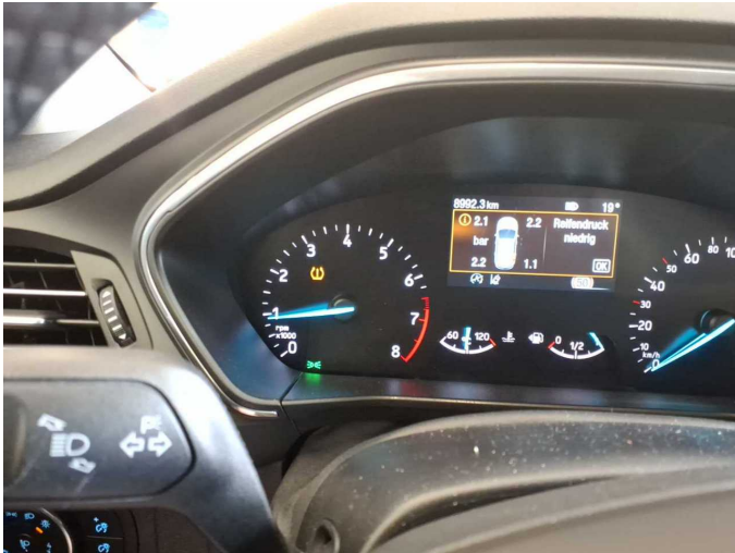
Damage 1: Instrument panel: Indicator light (Reifendruckkontrolle) - on - Perform diagnosis
