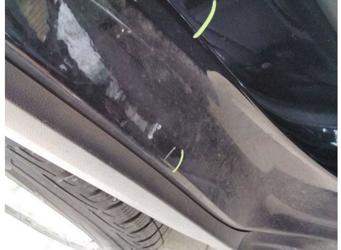
Damage 1: Body: C-pillar - right side - Scratch(es) - Smart repair
