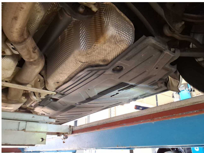
Damage 7: Body: Underbody panelling (rechts) - Broken / torn - Replace
