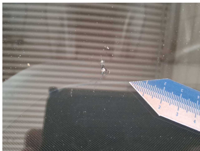
Damage 13: Vehicle glazing: Windscreen with lane departure assistant - Stone chips - Replace
