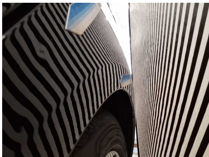
Damage 5: Side panel - rear left side: Side panel - dent(s) - Smart repair
