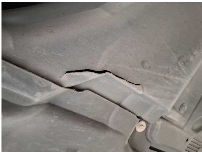
Damage 4: Mudguard - left side: Inner mudguard - Broken / torn - Replace
