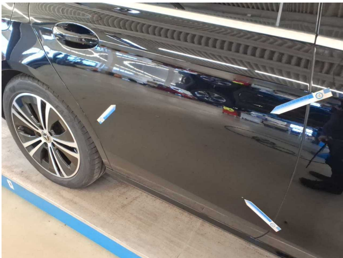
Damage 9: Door - rear right side: Door - Scratch(es) - Paint
