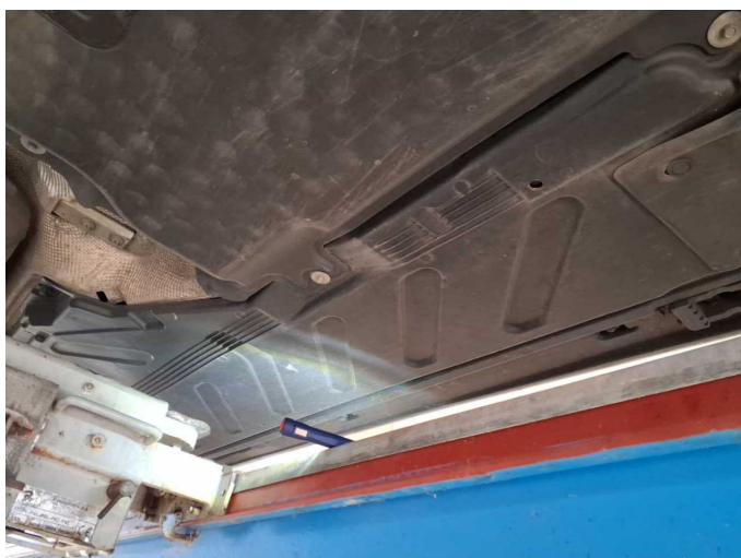
Damage 6: Body: Underbody panelling (links) - Broken / torn - Replace
