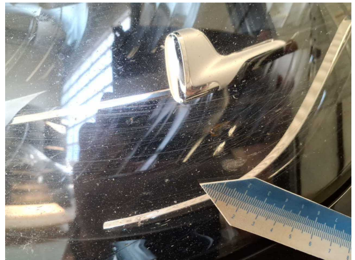
Damage 14: Headlight: Headlight - left side (+ rechts) - Scratched - Replace
