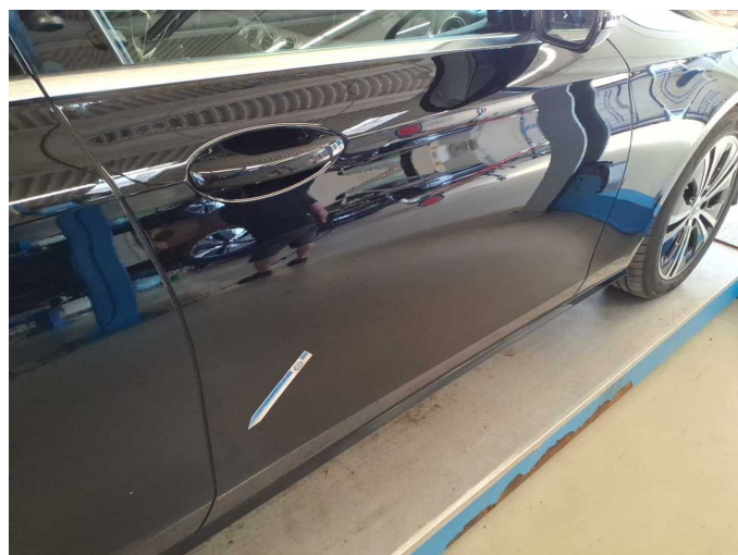
Damage 11: Door - front right side: Door - dent(s) - Repair and paint
