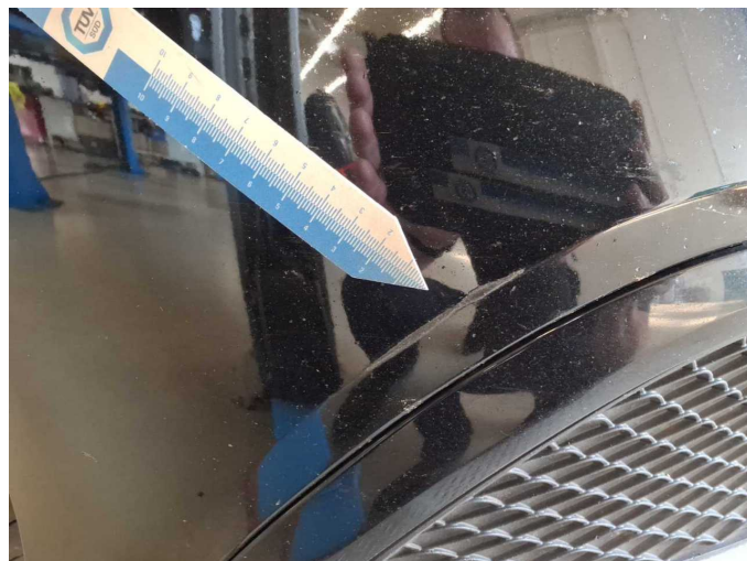
Damage 10: Front bumper: Bumper with Parktronic - Scratched - Paint
