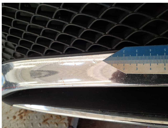
Damage 8: Trim / covers: Brightware / decorative strip (Stossfänger vorn) - Damaged - Replace
