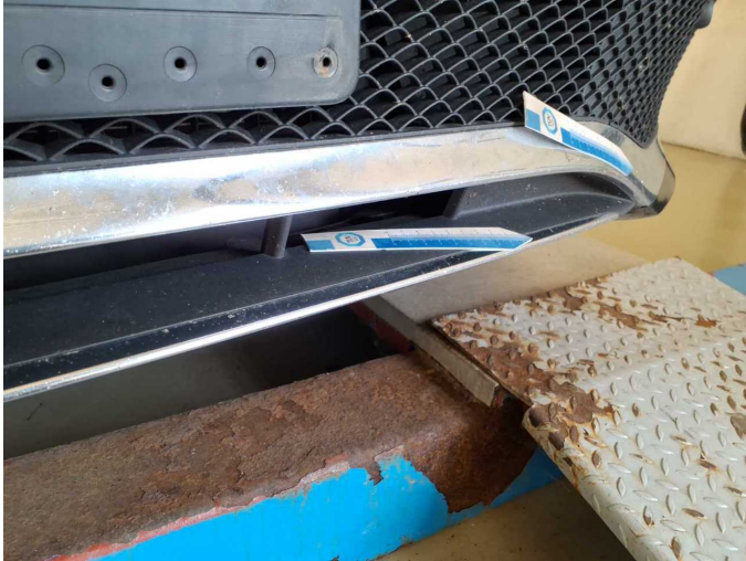
Damage 8: Trim / covers: Brightware / decorative strip (Stossfänger vorn) - Damaged - Replace
