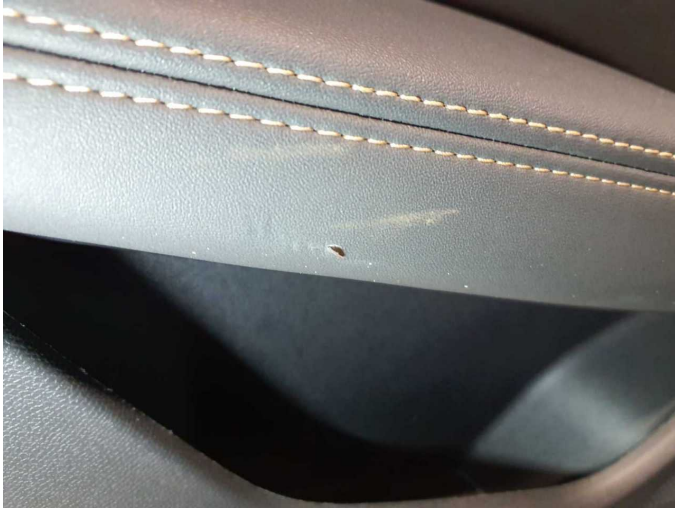
Damage 4: Trim / covers: Door trim - rear left side - Scratch(es) - Smart repair
