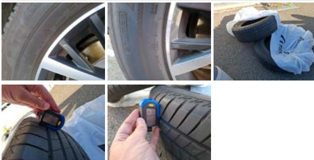
Tyre FL, Out of tolerance, Replace
