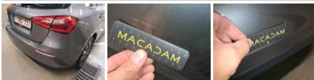
Roof pillar R, Dent(s), Acceptable
