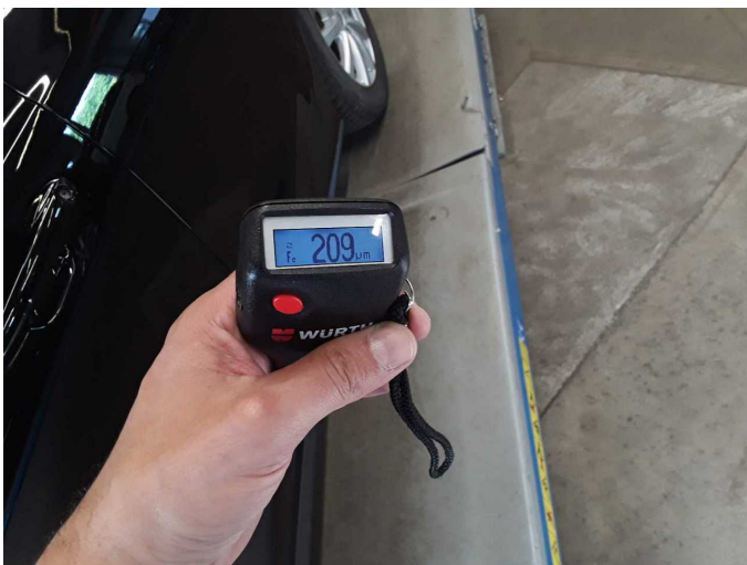
Repainting 1: Door - front left side
