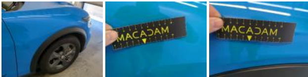
Door FR, Scratch(es), Repair and paint (complete)
