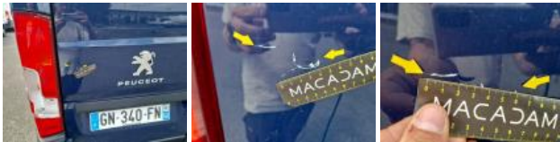
Bodywork, Glue residues, Remove lettering
