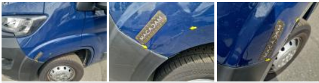
Side repeater L, Broken, Replace
