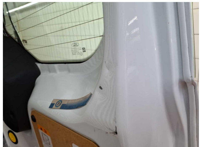
Damage 8: Boot lid / rear door: Rear door - right side - Dent / paintcoat damage - Repair and paint
