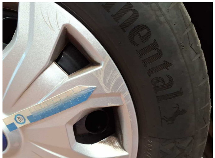
Damage 2: Wheel / tyres: Wheel cover - front left side - Scratched - Replace
