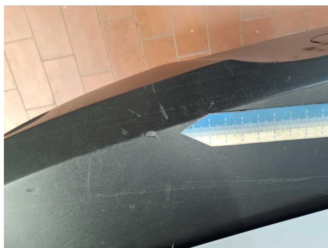
Damage 6: Rear bumper: Rear bumper - Scratch(es) - Replace
