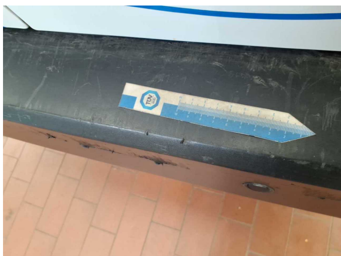
Damage 6: Rear bumper: Rear bumper - Scratch(es) - Replace
