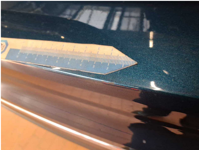
Damage 6: Rear bumper: Rear bumper - Scratch(es) - Paint
