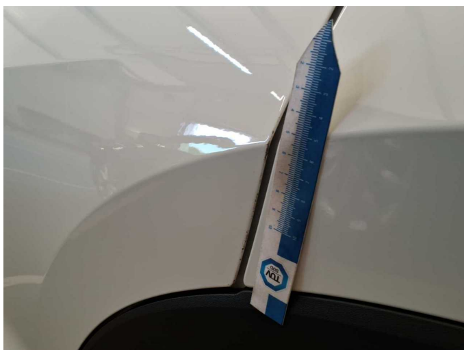
Damage 2: Door - rear left side: Door edge - Scratched - Smart repair
