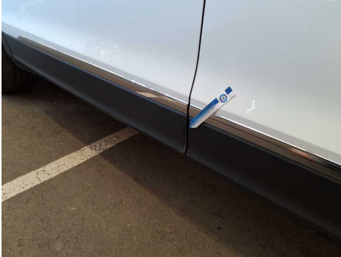
Damage 4: Door - front left side: Brightware - lower - Scratched - Replace
