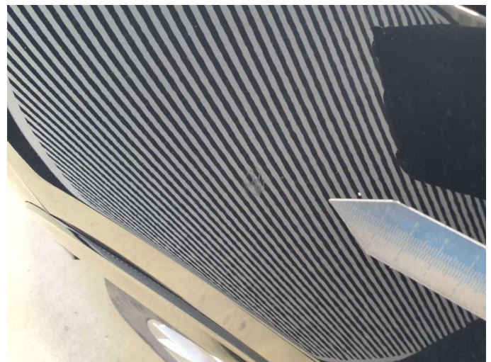
Damage 9: Mudguard - left side: Mudguard - left side (Spachtel eingefallen) - Unprofessionally repaired - Repair and paint
