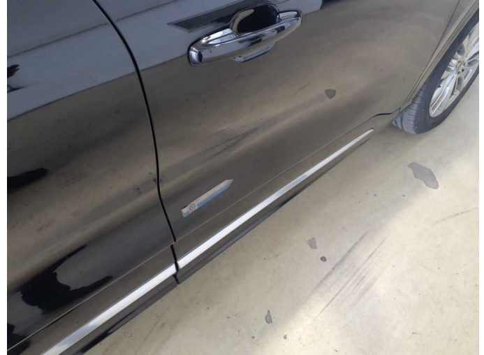
Damage 8: Door - front right side: Door - Dent / paintcoat damage - Smart repair
